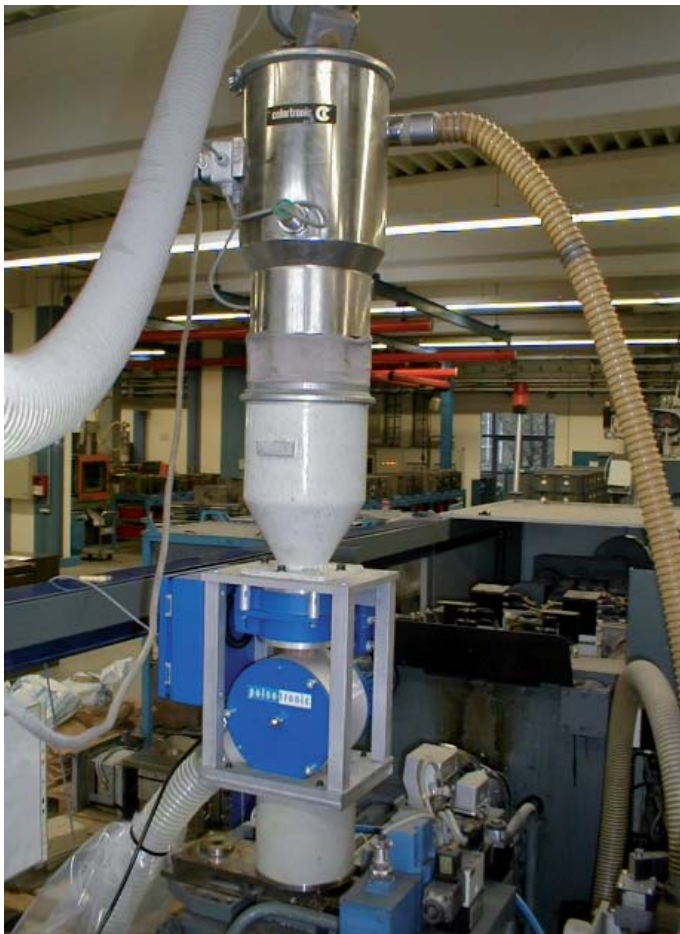
Digital Y 70 for the inspection of granulates in the plastics industry
